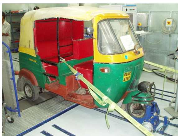
Figure 8: Autorickshaw on chassis dyno
