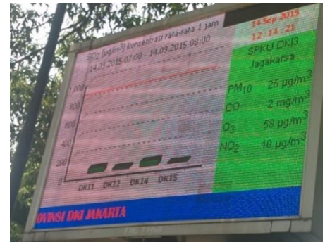
Electronic board showing the air quality levels from DKI 3 monitoring station
