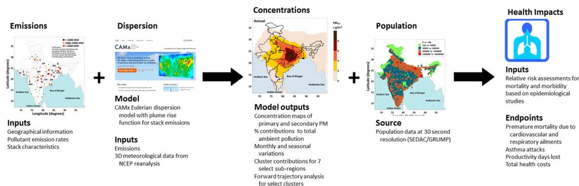
The atmospheric dispersion modeling of the emissions from all the coal-fired TPPs was conducted, following the above schematic and using the ENVIRON - Comprehensive Air Quality Model with Extensions (CAMx), an Eulerian photochemical dispersion model, suitable for integrated assessments of gaseous and particulate air pollution. The model formulation, advection and scavenging schematics, chemical solvers, and gas-to-aerosol conversion mechanisms<sup>17</sup>.
