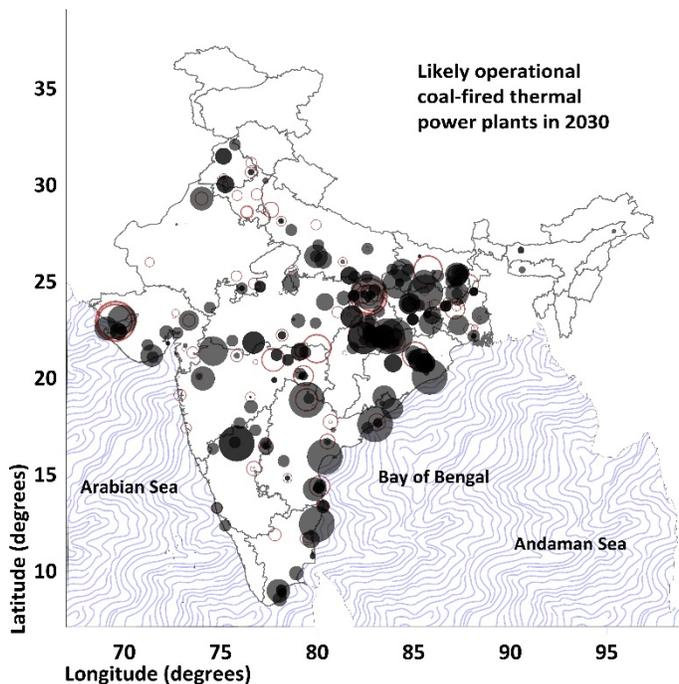
Clusters of coal-fired thermal power plants in 2030. The brown circles represent the thermal power plants operational in 2014 and the second colour represents all the expansions likely to be operational in 2030. The largest circle is 4620MW. Note that many of these circles are overlapping due to their close proximity
