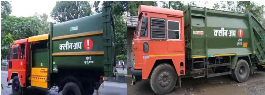
Side Loading Compactor- introduced for first time in India
